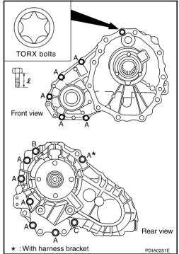
Separate front case and rear case. Then, remove front case by levering it up with a tire lever or the like.
