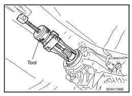
3. Put matchmark on the end of the mainshaft. The mark should be in line with the mark on the companion flange. CAUTION:
