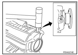
3. Install rear bearing to rear case, using a drift.
