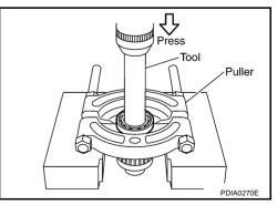
Remove front drive shaft front bearing, using drift and puller.
